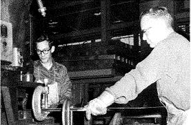
A sheet of steel is fed into a coping machine in the Dustube Fabrication section of the Steel Shop by Clay Spradlin, left, and John Fassero.
