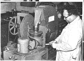
Long life characteristics of abrasives are checked in the life tester being demonstrated above.
